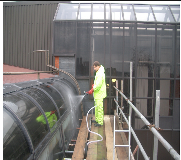
AAMA water spray testing of cladding
